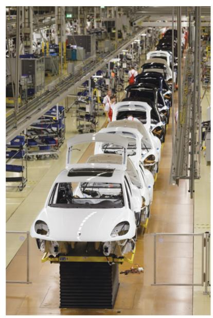
Energy saving: The lights are dimmed during the breaks at the Leipzig plant and the robots are switched off
